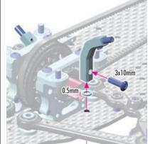
Attach the shock holder to both the chassis and bulkhead
