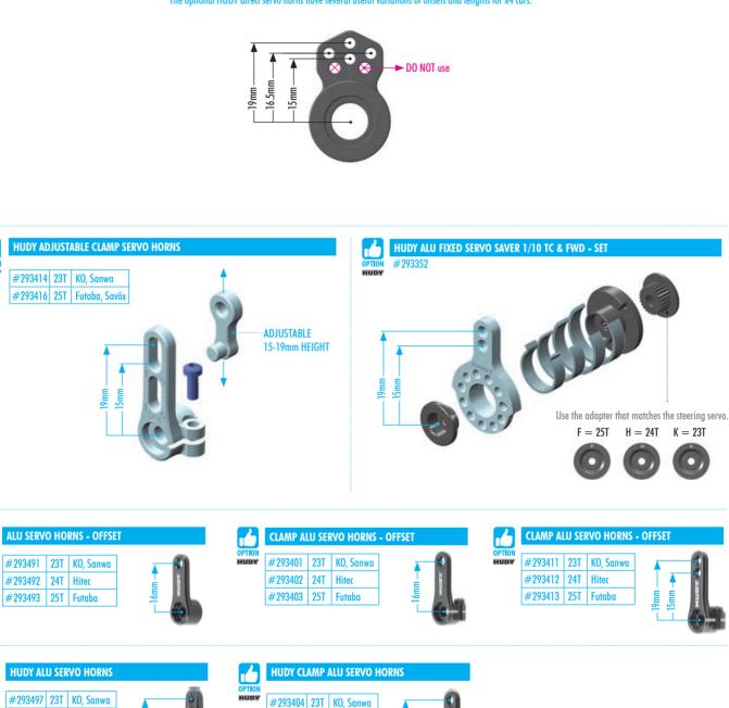
LONGER SERVO HORN LENGTH: Less servo rotation needed to reach the full steering lock, resulting in more responsive and immediate reaction to driver input. A servo horn that is too long can make the car feel nervous to drive. Most XRAY drivers prefer the 19mm length (top row on kit servo saver or 2nd hole on optional 2-hole alum horn).
