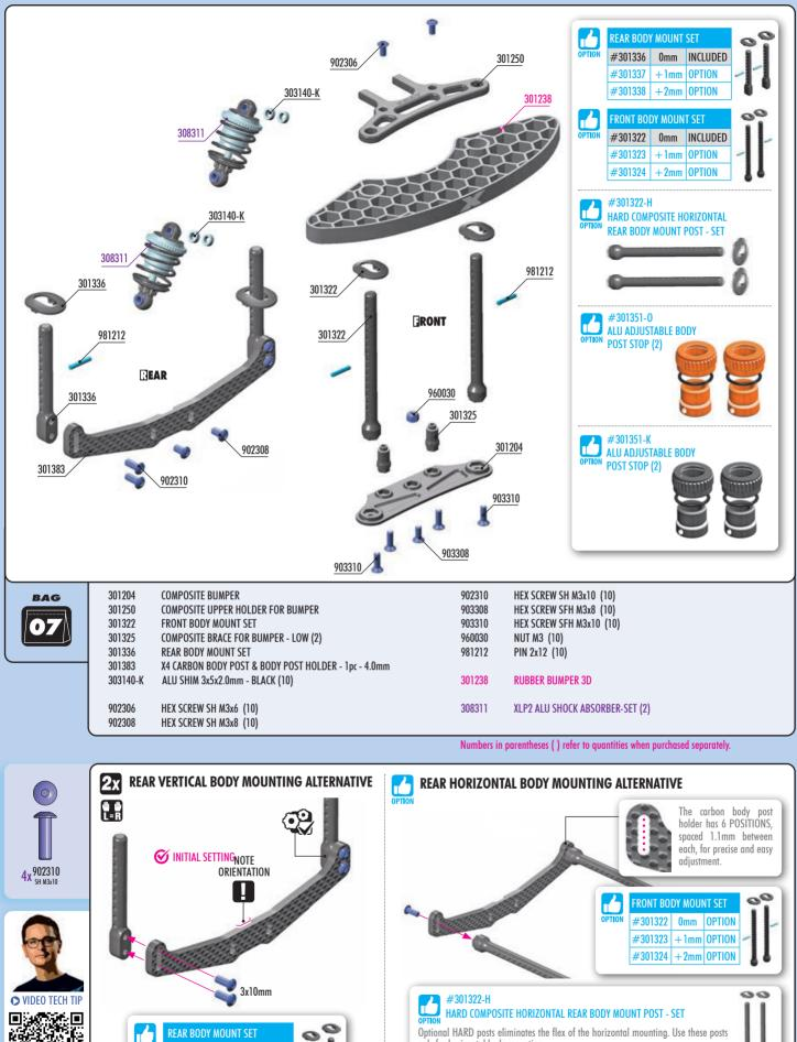
Optional HARD posts eliminates the flex of the horizontal mounting. Use these posts only for horizontal body mounting.
