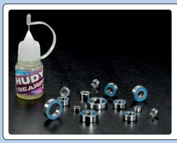
All ball-bearings are factory pre-oiled. Regularly service, clean and lubricate all ball-bearings with HUDY Bearing Oil (#106230). Replace any bearings that develop a "gritty" feeling to prevent inefficiency and avoid rear axle bearing blowouts.
