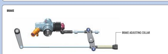
Adjust the composite collar on the brake linkage so the brakes work smoothly.
