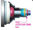
The clutch gap is A - B; the correct gap is 0.6-0.7mm
