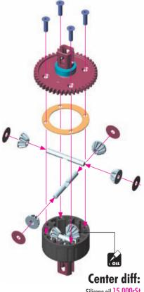
Silicone oil 15.000cSt Fill to just above the satellite gears.
