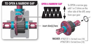
CHECK GEAR MESH AND DIFF PLAY ONLY AFTER THE ENTIRE GEARBOX IS MOUNTED TOGETHER WITH THE SUSPENSION HOLDERS ON THE CHASSIS. ALL PARTS ARE DESIGNED TO HAVE CERTAIN PLAY AND IT IS ALL DESIGNED BY PURPOSE.
