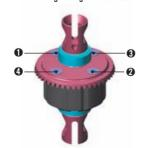
After assembly the differentials should have a length of 32.3~32.5 mm measured from the ends of the installed ball-bearings. If differentials are longer, retighten the 4 screws holding the crown gears.
