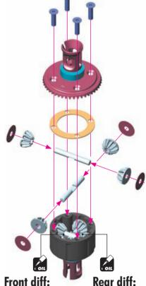
Silicone oil 10.000cSt Fill just above the satellite gears.
