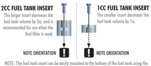
provided screw, when the fuel tank cap is opened fully.
