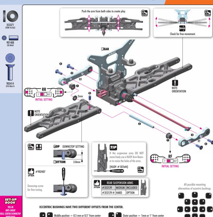
The XRAY rear alu lower suspension holders provide even greater range of adjustment for the rear suspension. Using different combinations of eccentric bushings, fine adjustment of rear anti-squat, rear toe-in, rear roll center, and rear track-width can be obtained. For more information about the influence of rear anti-squat, rear toe-in, rear roll center and rear track-width on car handling, please refer to HUDY Off-Road Set-up Book (#209099).
