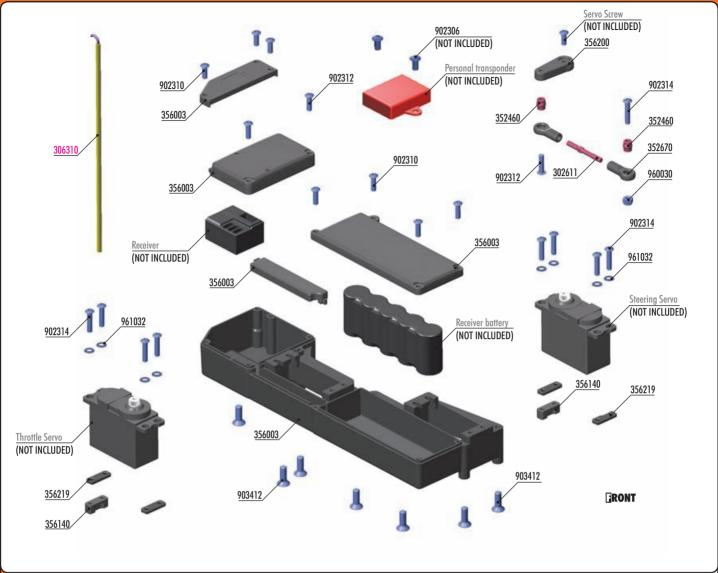
BAG 10 302611 ADJ. TURNBUCKLE L/R 35 MM - HUDY SPRING STEEL™ (2) PIVOT BALL 5.8 (10) SERVO BALL JOINT 5.8MM (4) 352460 352670 356003 COMPOSITE RADIO CASE SET - HARD BATTERY CABLE WITH SWITCH (OPTION) 356050 COMPOSITE SERVO MOUNT - SMALL (2) 356140 356200 BRAKE/THROTTLE ARMS & STEERING SERVO ARMS - SET COMPOSITE SERVO SHIMS 1.0, 1.5 & 2.5MM (2+2+2) 356219 389135 CONNECTING CABLE RECEIVER/BATT. PACK (OPTION)
