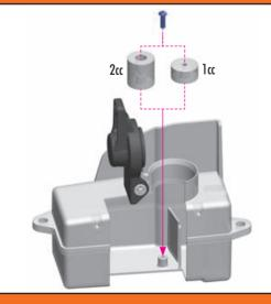
The fuel tank has the larger fuel volume and includes OPTIONAL tank inserts for decreasing the volume of the tank. Using the inserts allows you to adjust the volume of fuel inside the tank; this works in conjunction with variables such as fuel filter capacity and/or length of fuel line to ensure you have the legal fuel volume limit for racing.
