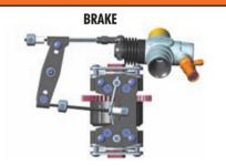
Adjust the adjustable collars so the brakes work smoothly. If the brakes apply too much or not enough, adjust the adjustable collars accordingly. Or if available on the transmitter, adjust the brake endpoint. To tighten brakes, turn collar to thread brake rod INTO pivot. To loosen brakes, turn collar to thread brake rod OUT of pivot.
