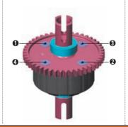
After assembly the differential should have a length of 32.3~32.5 mm measured from the ends of the installed ball-bearings. If differential is longer, retighten the 4 screws holding the spur gear.
