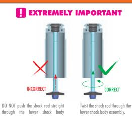
assembly; O-ring damage may result.
