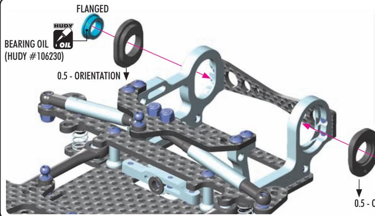
These eccentric bushings adjust the **RIDE HEIGHT** of the rear pod. Make sure to use the **SAME** eccentric bushings on **BOTH** sides.
