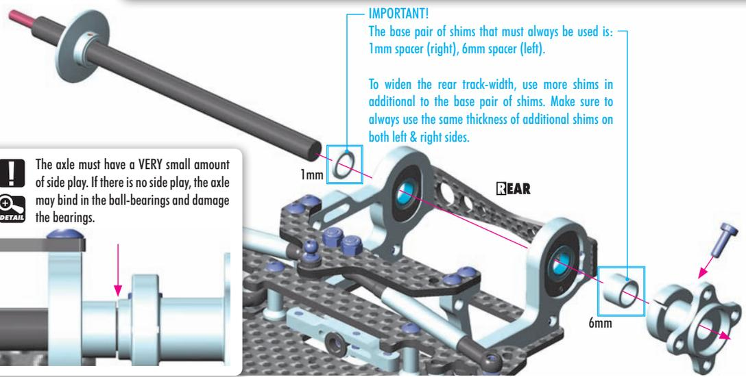
**!** The axle must have a **VERY** small amount of side play. If there is no side play, the axle may bind in the ball-bearings and damage the bearings.
