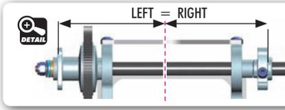
To set track-width, use the hole in the pod lower plate as the centre point; this hole should always be centred between the two rear wheels once overall track-width is set. To set the track-width more easily, set the car on a ruler or use a digital vernier caliper. Rear track-width is directly affected by wheel offsets, which can vary depending on tire brand.
