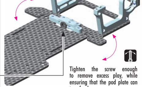
Tighten the screw enough to remove excess play, while ensuring that the pod plate can turn freely.
