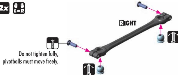
Do not tighten fully, pivotballs must move freely.
