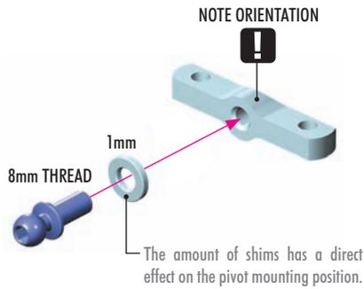
The amount of shims has a direct effect on the pivot mounting position.
