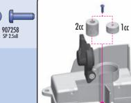
The fuel tank has the larger fuel volume and includes OPTIONAL tank inserts for decreasing the volume of the tank. Using the inserts allows you to adjust the volume of fuel inside the tank; this works in conjunction with variables such as fuel filter capacity and/or length of fuel line to
