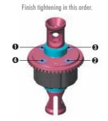
After assembly the differentials should have a length of  $32.3 \sim 32.5$  mm measured from the ends of the installed ball-bearings. If differentials are longer, retighten the 4 screws holding the crown gears.
