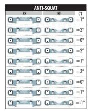
The new XRAY rear alu lower suspension holders provide even greater range of adjustment for the rear suspension. Using different combinations of eccentric bushings, fine adjustment of rear anti-squat, rear toe-in, rear roll center, and rear track-width can be obtained. For more information about the influence of rear anti-squat, rear toe-in, rear roll center and rear track width on car handling, please refer to HUDY Off-Road Set-up Book (#209099).
