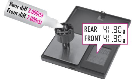
1. Put the diff (without oil) on the scale and check the weight:
