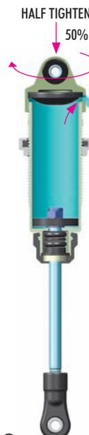
**5** Gently place the shock cap assembly onto the filled shock body. Excess oil will spill from the shock. Screw the shock cap onto the body by only a few turns.
