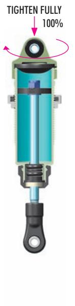
**7** Keep the shock shaft pushed in the shock body and tighten the shock cap completely. The rebound will be at approximately 0%.
