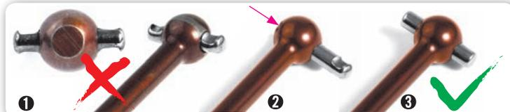
1 Do not use drive shafts when the pins are worn.
