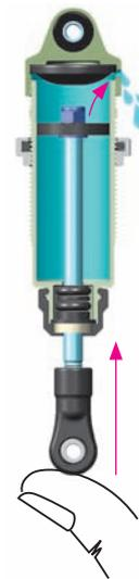
**6** Gently push the shock shaft completely into the shock body. Excess oil will flow through the hole in the shock cap.
