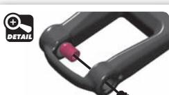
**TIP** Press pivot ball into arm until it snaps into place
