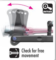
Do not overtighten the self-locking nut. Overtightening may result in suspension binding.
