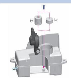
The fuel tank volume can be adjusted using the included inserts. The inserts reduce fuel capacity inside the tank to adjust for fuel filter and fuel line capacity and ensure a legal fuel volume for racing.
