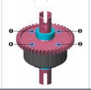
After assembly the differential should have a length of  $32.3 \sim 32.5$ mm measured from the ends of the installed ball-bearings. If the differential is longer, check that the gear is properly seated on the case and retigihten the 4 screws while holding the spur gear.
