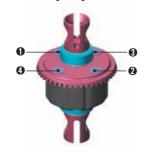
After assembly the differentials should have a length of 32.3~32.5 mm measured from the ends of the installed ball-bearings. If the differentials are longer, check that the gear is properly seated on the case and retighten the 4 screws while holding the crown gear.
