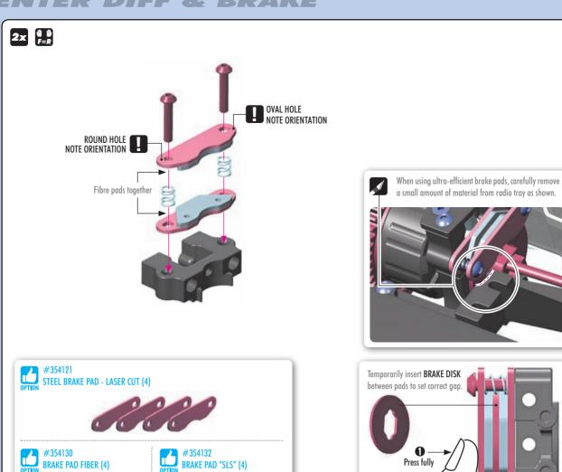
It is necessary to glue the brake pad with strong CA glue suitable for steel.
