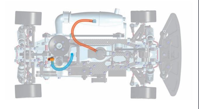
**ALTERNATIVE 2** Fuel tube routed from muffler into the fuel tank through 2 holders on radio tray.
