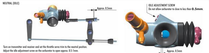
Adjust both collars on the carb and brake linkages accordingly. The carb linkage must have approximately 0.5mm of preload on the spring at neutral. DO NOT ADJUST while the engine is running.
