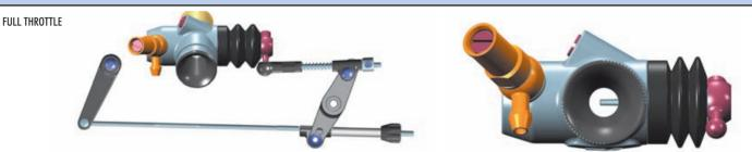
With the engine NOT RUNNING but the receiver turned ON, apply full throttle at the transmitter.
