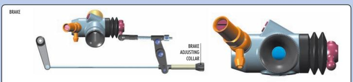
Adjust the composite collar on the brake linkage so the brakes work smoothly.
