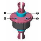
After assembly the differentials should have a length of 32.3~32.5 mm measured from the ends of the installed ball-bearings. If differentials are longer, retighten the 4 screws holding the crown gears.
