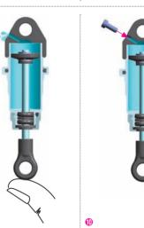
Tighten the screw. The rebound will be at approx. 0%
