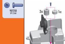
The fuel tank has the larger fuel volume and includes OPTIONAL tank inserts for decreasing the volume of the tank. Using the inserts allows you to adjust the volume of fuel inside the tank; this works in conjunction with variables such as fuel filter capacity and/or length of fuel line to ensure you have the legal fuel volume limit for racing.
