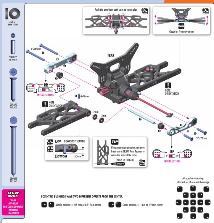
The new XRAY rear alu lower suspension holders provide even greater range of adjustment for the rear suspension. Using different combinations of eccentric bushings, fine adjustment of rear anti-squat, rear toe-in, rear roll center, and rear track-width can be obtained. For more information about the influence of rear anti-squat, rear toe-in, rear roll center and rear track width on car handling, please refer to HUDY Off-Road Set-up Book (#209099).
