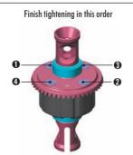
After assembly the differentials should have a length of  $32.3\sim32.5$  mm measured from the ends of the installed ball-bearings. If differentials are longer, retighten the 4 screws holding the crown gears.
