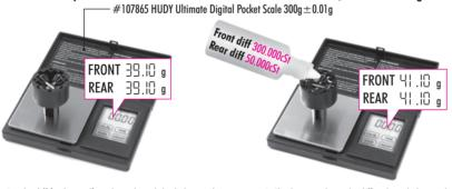
1. Put the diff (without oil) on the scale and check the weight: - FRONT DIFF approx. 39.10a
