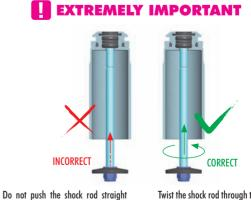
through the lower shock body assembly; O-ring damage may result.
