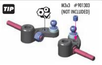
When using rearward hole, you can reinforce the steering block (for hard crashes) by installing an M3x3 setscrew in the forward hole.
