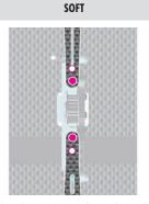
This allows maximum flex and provides maximum steering. However, the car is less stable on-power.
